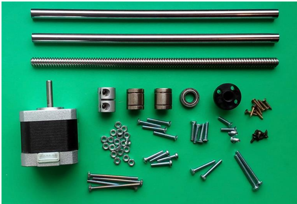
Fig. 6. Guide rods, lead screw with nut, metal rigid coupling, bearings, stepper motor, screws and nuts.
