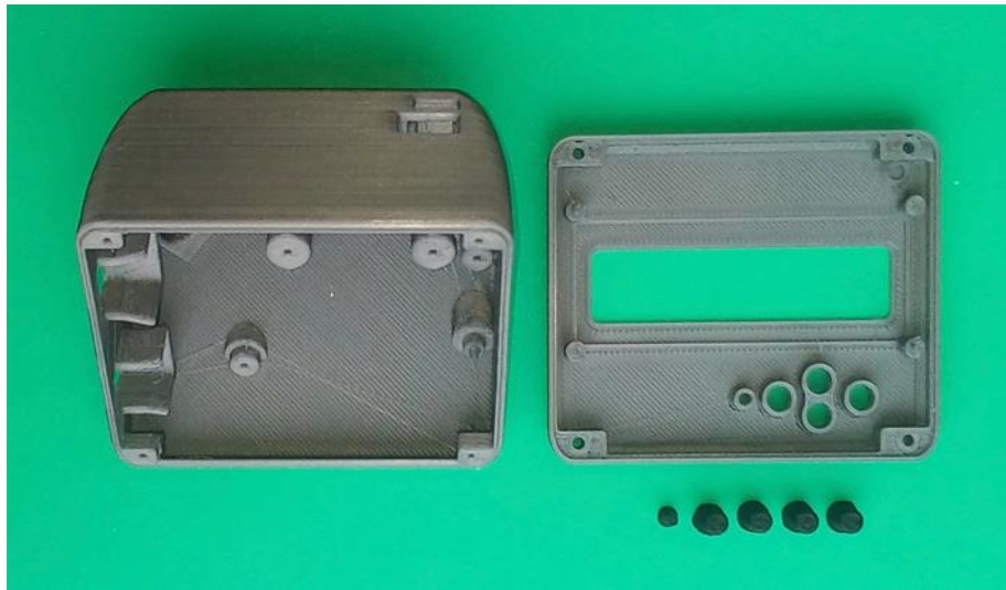
Fig. 5. Plastic case made on 3D printer.
